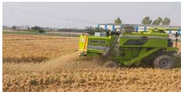
Figure 5. Super Straw Management System(SMS)machine while chopping and shredding the crop residues in the field creating a surface mulch
