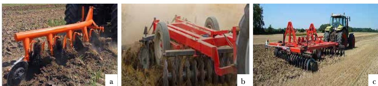
Figure 6. Incorporation of crop residues in field through different machineries. (a. Malboard plow, b. Disk c. Harrow)
